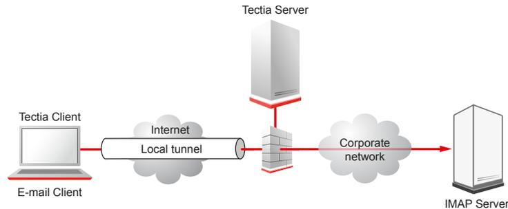
**Figure 6.1. Local tunnel to an IMAP server**
